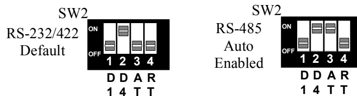
Figure 6 - RS-485 Enable modes
